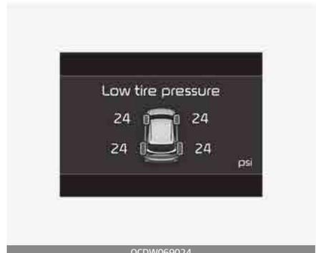
When the tire pressure monitoring system warning indicators are illuminated and warning message displayed on the cluster LCD display, one or more of your tires is significantly under-inflated. The low tire pressure position telltale light will indicate which tire is significantly under-inflated by illuminating the corresponding position light.
