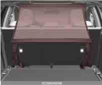
It is designed to help protect the heads of the occupants by preventing objects from flying forward in frontal collisions.
