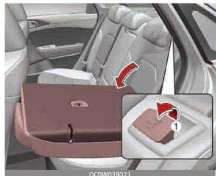
3. On rear outboard seatback: Pull the lock release lever (1) and fold
