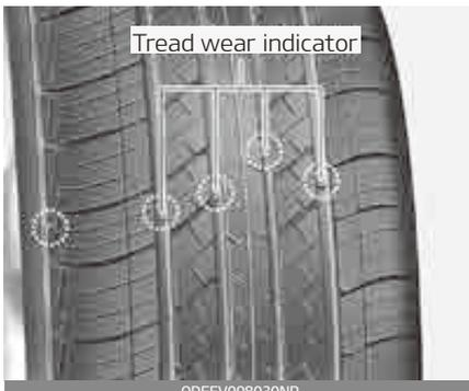
This shows there is less than 1.6 mm (1/16 in.) of tread left on the tire. Replace the tire when this happens.
