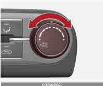
To change the air temperature in the passenger compartment:
