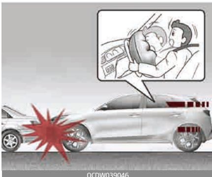
Front air bags are designed to inflate in a frontal collision depending on the intensity, speed or angles of impact of the front collision.
