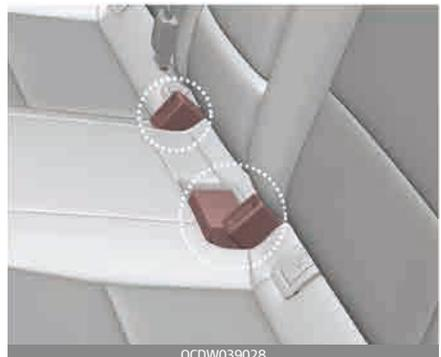
The rear seat belt buckles can be stowed in the pocket between the rear seatback and cushion when not in use.
