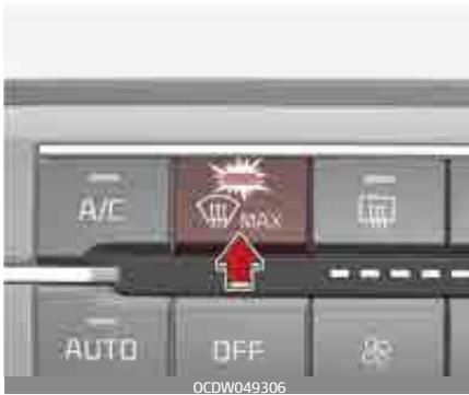
When you select the defrost mode, the following system settings will be made automatically:
