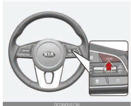
1. Press the CRUISE button on the steering wheel, to turn the system on. The set speed will illuminate.
