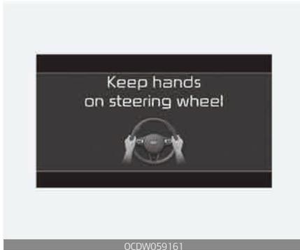
If you keep your hands off the wheel while driving with the LFA system assisting the steering, the hands-off warning will be triggered.
