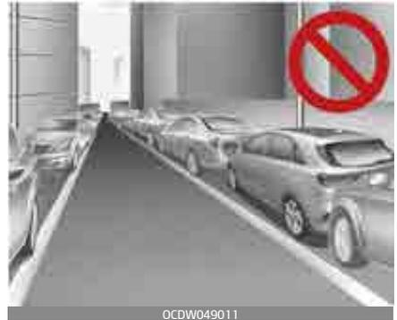
When leaving a parking space that is narrow and near a wall, the system may not work properly. When leaving a parking space similar to the above picture, the driver must watch out for obstacles while leaving.
