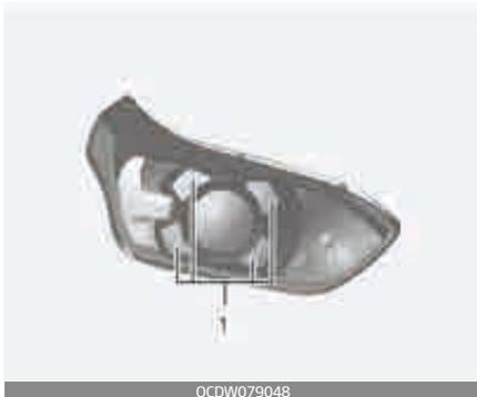
If the position lamp + DRL (LED) (1) does not operate, have your vehicle checked by a professional workshop.
