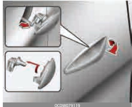
1. Remove the lamp assembly from the vehicle by prying the lens and pulling the assembly out.
