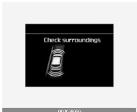
The Parking Assist checks the front and rear space to exit the vehicle from the parking space.
