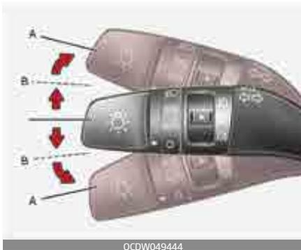
The ignition switch must be on for the turn signals to function. To turn on the turn signals, move the lever up or down (A).
