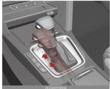
Whether the vehicle is stationary or in motion, sports mode is selected by pushing the shift lever from the D (Drive) position into the manual gate. To return to D (Drive) range operation, push the shift lever back into the main gate.
