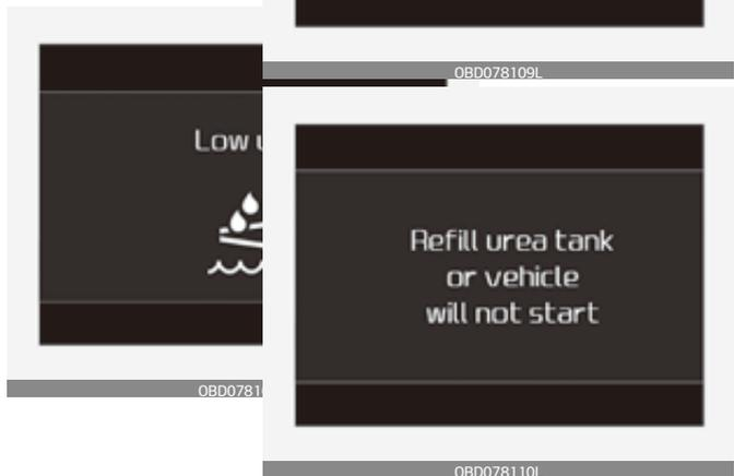
The lack warning messages of urea solution appear below urea solution approximately 3.6 L. When the warning message "Low Urea" is displayed with SCR warning lamp (
