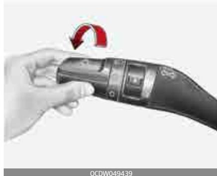
When the light switch is in the parking light position (2nd position), the tail position, license and instrument panel lights will turn ON.
