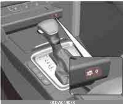
Firmly close all doors, and turn the ignition to ACC or IGN ON. To start wireless charging, place the smart phone equipped with wireless
