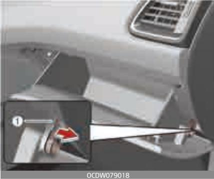
3. Remove the climate control air filter cover by pulling out both sides of the cover.
