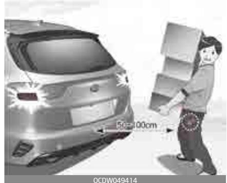
If you are positioned in the detecting area (50 ~100 cm behind the vehicle) carrying a smart key, the hazard warning lights will blink and chime will sound for about 3 seconds to alert you the smart key has been detected and the tailgate will open.
