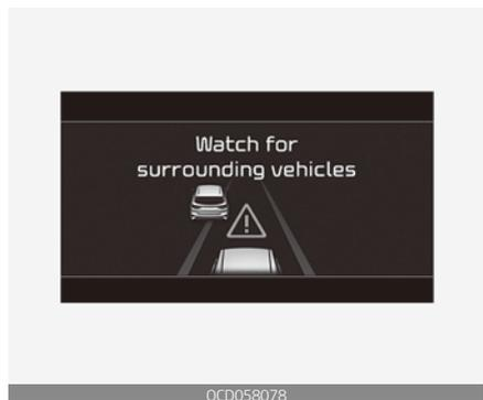
If the vehicle ahead (vehicle speed: less than 30km/h) disappears to the next lane, the warning chime will sound and a message will appear. Adjust your vehicle speed for vehicles or objects that can suddenly appear in front of you by depressing the brake pedal according to the road condition ahead and driving condition.
