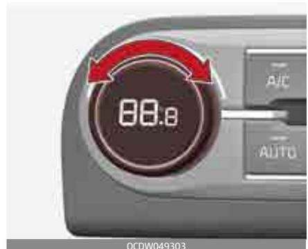
The temperature will increase to the maximum (HI) by turning the knob to the right extremely.
