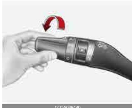
When the light switch is in the headlight position (3rd position), the head, tail, position, license and instrument panel lights are ON.
