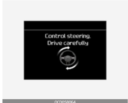
When assisting the driver exit the parking space is completed the above message will appear.
