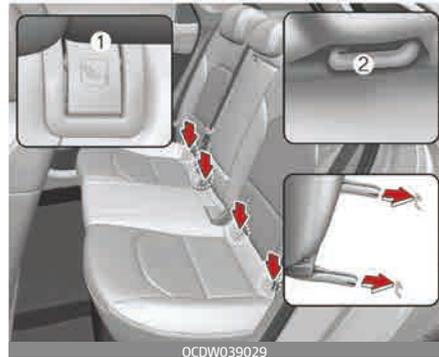
ISOFIX(i-Size) anchorages are located between the seatback and the seat cushion of the rear seat left and right outboard seating positions, indicated by the symbols.
