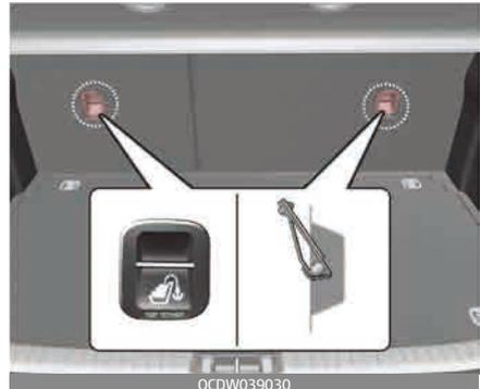
Child restraint system top tether anchorages are located on the back of the rear seatbacks.
