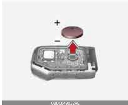
The transmitter uses a 3 volt lithium battery which will normally last for several years. When replacement is necessary, use the following procedure.
