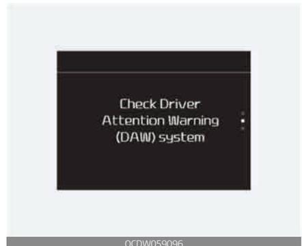
When the "Check System" warning message appears, the system is not working properly. In this case, we recommend you to have the vehicle inspected by an authorized Kia dealer.
