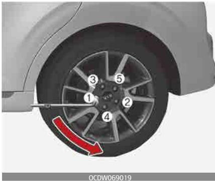
6. Loosen the wheel lug nuts counterclockwise one turn each, but do not remove any nut until the tire has been raised off the ground.
