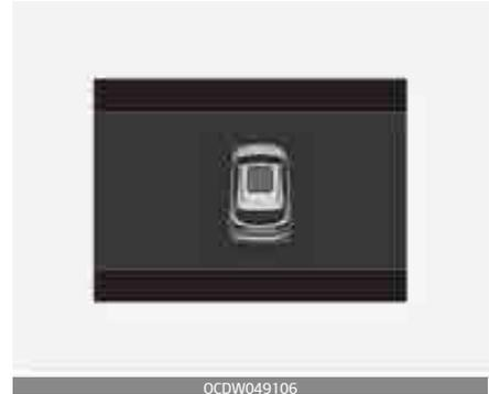
If the driver removes the ignition key (smart key: turns off the engine) when the sunroof is not fully closed, the warning chime will sound for a few seconds and a warning image will appear in the LCD window. Close the sunroof securely when leaving your vehicle.
