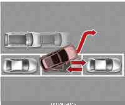
The Parking Assist helps drivers park their vehicle by using sensors to measure parking spaces, control the steering wheel to semi-automatically park the vehicle and provide instruction on the LCD display to help through parking.
