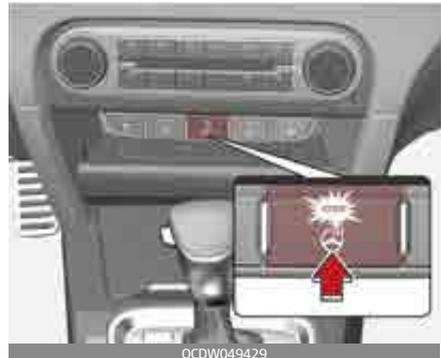
When the ignition switch is in the ON position, pressing the heated steering wheel button warms the
