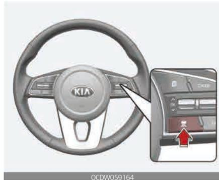
This function allows you to program the vehicle to maintain relative distance to the vehicle ahead without depressing the accelerator pedal or brake pedal.
