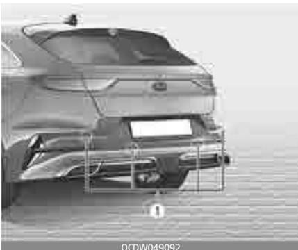
The parking distance warning assists the driver during movement of the vehicle by chiming if any object is sensed within the distance of 105 cm (41 in.) in front and 125 cm (49 in.) behind the vehicle.
