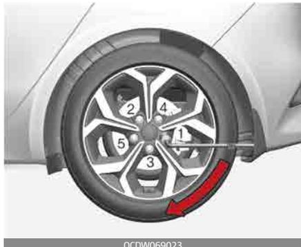
Then position the wrench as shown in the drawing and tighten the wheel nuts. Be sure the socket is seated completely over the nut. Do not stand on the wrench handle or use an extension pipe over the wrench handle. Go around the wheel tightening every other nut until they are all tight. Then double-
