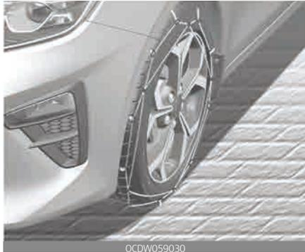
Since the sidewalls of radial tires are thinner, they can be damaged by mounting some types of snow chains on them. Therefore, the use of snow tires is recommended instead of snow chains. Do not mount tire chains on vehicles equipped with aluminum wheels; snow chains may cause damage to the wheels. If snow chains must be used, use wire-type chains with a thickness of less than 12 mm (0.47 in). Damage to your vehicle caused by improper snow chain
