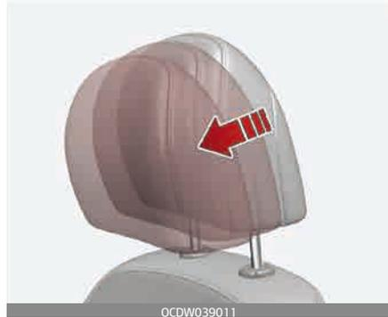
The headrest may be adjusted forward to 4 different positions by pulling the headrest forward to the desired detent.
