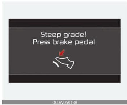
This warning message is displayed when vehicle is driven slowly on a grade and the vehicle detects that the brake pedal is not applied.
