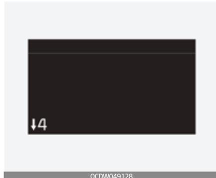
In the Manual shift mode, this indicator informs which gear is desired while driving to save fuel.
