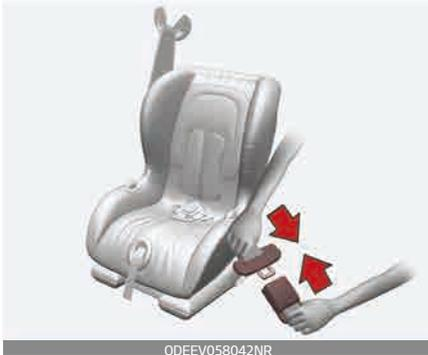
3. Remove as much slack from the belt as possible by pushing down on the Child Restraint System while feeding the shoulder belt back into the retractor.
