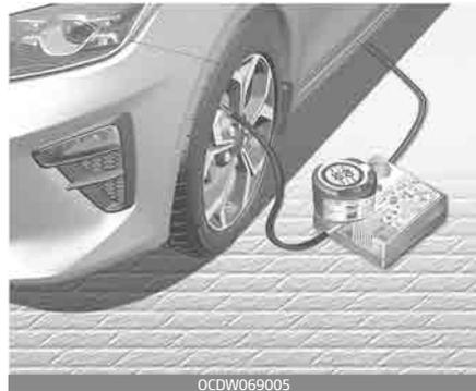
8. Ensure that the compressor is switched off, position 0.
