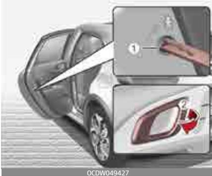
If children accidentally open the rear doors while the vehicle is in motion, they could fall out and be severely injured or killed. To prevent children from opening the rear doors from the inside, the rear door safety locks should be used whenever children are in the vehicle.
