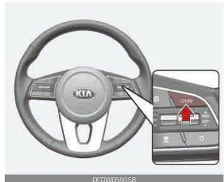
1. Press the CRUISE button, to turn the system on. The CRUISE indicator in the instrument cluster will illuminate.
