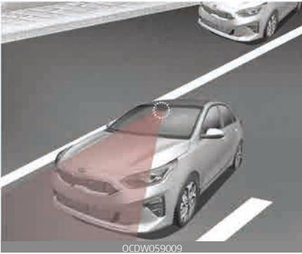
The Lane Following Assist System is designed to center the vehicle in the chosen lane by using a front mounted camera on top of the windshield.
