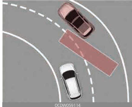
The BCW systems may not operate properly when driving on a curved road. In certain instances the system may not detect the vehicle in the next lane.
