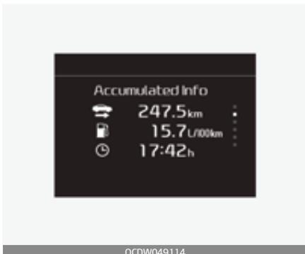
Displays accumulated information starting from mileage/fuel efficiency/time default point.
