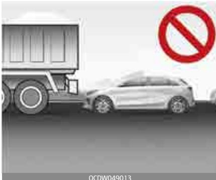
An accident may occur when parking behind a vehicle higher than yours. For example, bus, truck, etc.
