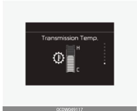
This mode displays the transmission temperature.
