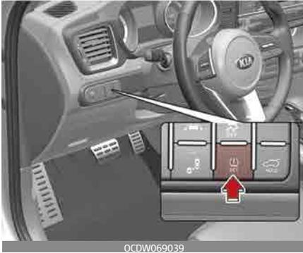
4. Then check that the low tire pressure indicator turns off after blinking for four seconds. In case of supervision cluster, check that "Tire pressures stored" message is shown on the cluster.
