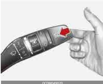
In the OFF (O) position, pull the lever gently toward you to spray washer fluid on the windshield and to run the wipers 1-3 cycles.
