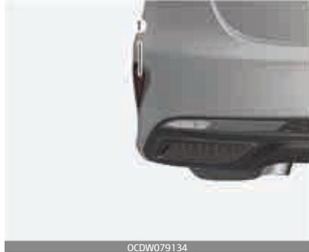
If the rear fog lamp (LED) (1) does not operate, have your vehicle checked by a professional workshop.
