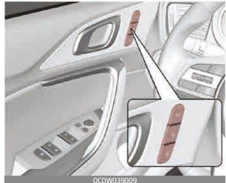
A driver position memory system is provided to store and recall the driver seat position with a simple button operation. By saving the desired position into the system memory, different drivers can reposition the driver seat based upon their driving preference. If the battery is disconnected, the position memory will be erased and the driving position should be restored in the system.
