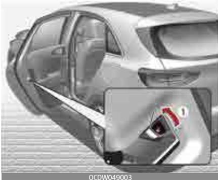
If the power door lock switch does not operate electrically, the only way to lock the door(s) is with the mechanical key from the outside key hole.
