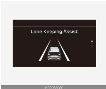
If the speed of the vehicle is over 60 km/h (37 mph) and the system detects lane markers, the color changes from gray to white.
