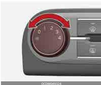
The fan speed control knob allows you to control the fan speed of the air flowing from the ventilation system.
