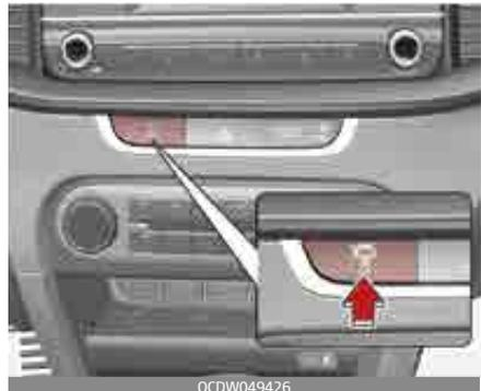
It is operated by pressing the door lock/unlock switch.
