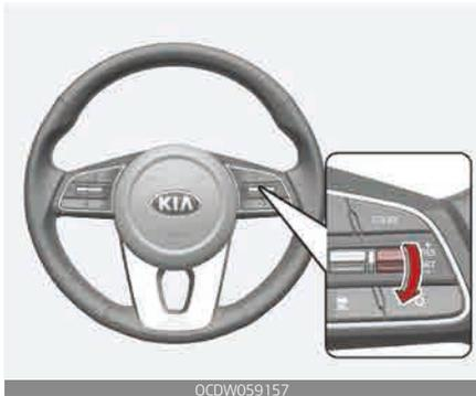
3. Move the lever down (to SET-), and release it at the desired speed. The cruise set speed will illuminate. Release the accelerator pedal at the same time. The desired speed will automatically be maintained.
