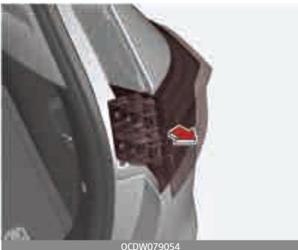
4. Remove the rear combination lamp assembly from the body of the vehicle.
