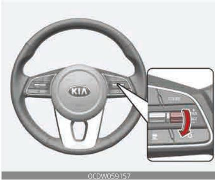
3. Move the lever down (to SET-), and release it at the desired speed. The set speed and vehicle to vehicle distance on the screen will illuminate.
