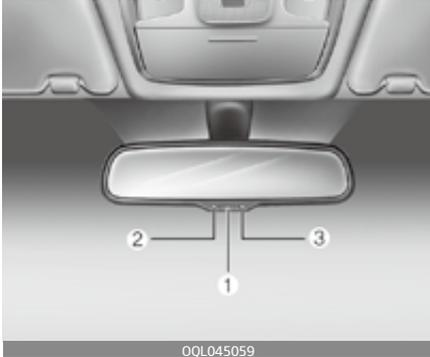
The electric rear view mirror automatically controls the glare from the headlights of the vehicles behind you in nighttime or low light driving conditions. The sensor (3) mounted in the mirror senses the light level around the vehicle, and automatically controls the headlight glare from the vehicles behind you.
