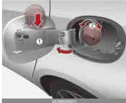
2. Pull the fuel filler door (1) out to fully open.
